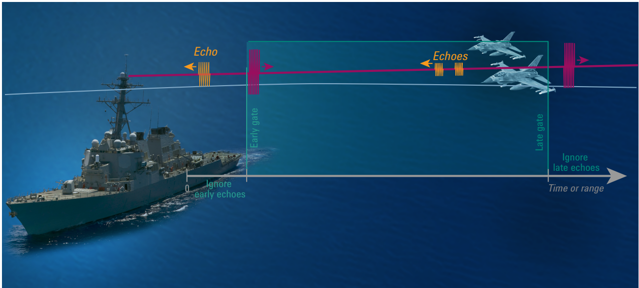
Figure 3. Time gating or range gating
