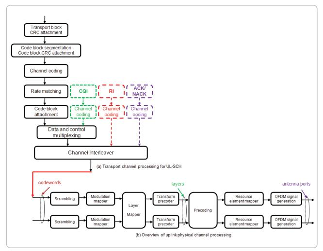
Figure 11. Uplink channel coding (TS 36.212) and physical channel processing (TS36.211) [ref 3,4, 16]
