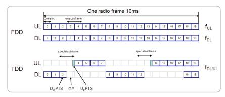
Figure 1. LTE FDD/TDD frame structure (Parkvall & Astely, pp 148 [14])
