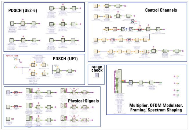
Figure 18. Schematic of LTE-Advanced DL MIMO source, underneath the symbol in Figure 17. This network is parameterized and wrapped under a more convenient GUI, shown in Figures 19-24.
