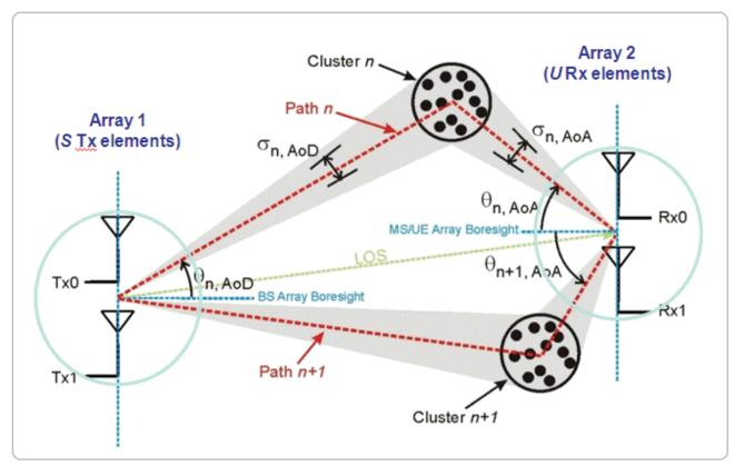
Figure 14. Representation of the MIMO channel
