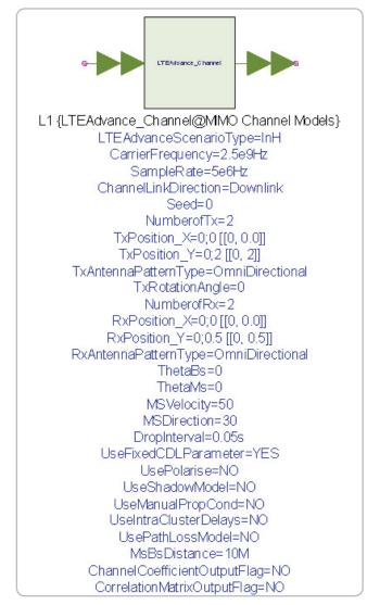
Figure 37. LTE-Advanced MIMO channel model in SystemVue
