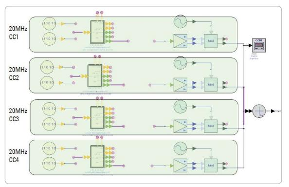
Figure 41. Schematic of scenario 1, 4x20MHz carrier aggregation in SystemVue
