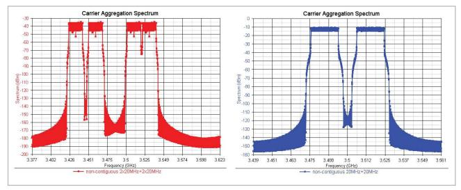
Figure 43. Spectrums of scenario 4 with non-contiguous CCs. (a) is the spectrum of DL (2x20 + 2x20MHz CCs) and (b) is the spectrum of UL (1x20 + 1x20MHz CCs)
