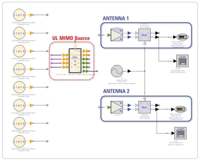
Figure 44. Schematic of clustered DFT-S-OFDM
