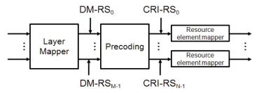
Figure 13. DMRS-based MIMO scheme in LTE-Advanced
