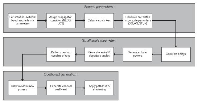
Figure 16. Procedure for generating channel coefficient [TR 36.814]
