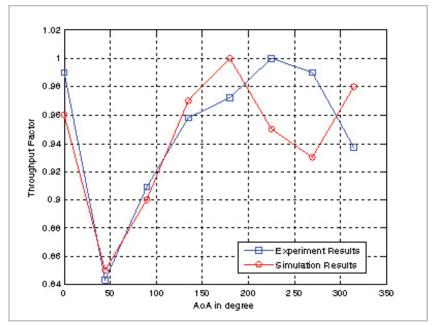
Figure 47. LTE-Advanced throughput vs. Angle of Arrival (AoA), measured vs. simulated results
