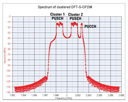
Figure 45. Spectrum of clustered DFT-S-OFDM in SystemVue
