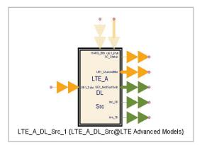
Figure 17. Downlink MIMO Source in the SystemVue LTE-Advanced library
