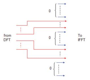
Figure 8. Mapping function of clustered SC-FDMA
