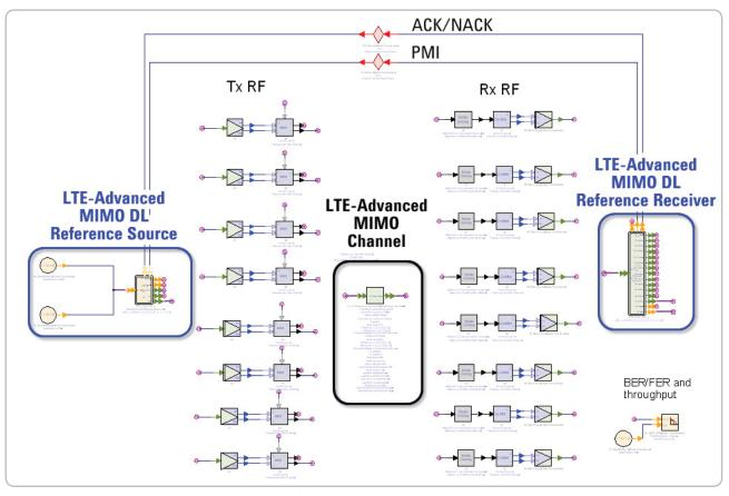
Figure 46. Schematic of the LTE Advanced DL 8X8 MIMO scenario, with fading and closed-loop throughput measurement with active HARO feedback. SystemVue's "dynamic dataflow" technology is critical for performing this virtual OTA simulation.
