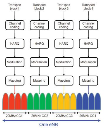
Figure 5. Carrier allocation in contiguous DL carrier aggregation [15]
