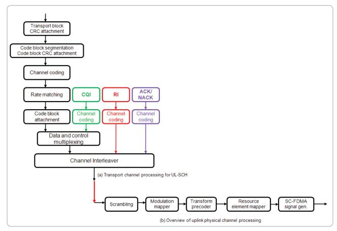
Figure 3. Uplink channel coding (TS 36.212) and physical channel processing (TS36.211) [ref 3,4, 16]
