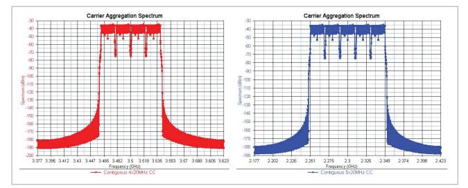
Figure 42. Spectrums of downlink contiguous CCs. (a) is the spectrum of scenario 1 (4x20MHz CCs) and (b) is the spectrum of scenario 2 (5x20MHz CCs)
