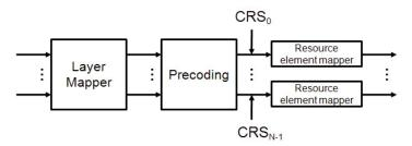
Figure 12. CRS-based MIMO scheme in LTE
