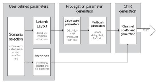
Figure 15. Process for creating generic channel model [TR 36.814]
