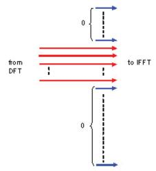
Figure 7. Subcarrier mapping for SC-FDMA
