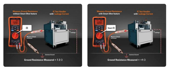
Note: The maximum correctable offset/bias voltage is +50 mV / -30 mV for the 30  $\Omega$  range and +1.0 V / -0.2 V for the 300  $\Omega$ , 3 k $\Omega$ , 30 k $\Omega$ , and 300 k $\Omega$  ranges. If the dc voltage on the resistor is over the maximum correctable offset/bias voltage, the OL sign is shown on the secondary display.
