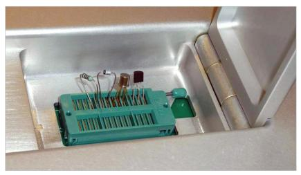
*Figure 4. Using a MUX, students can remotely switch between devices under test. From left to right: resistor, diode, mosfet, and bipolar transistor*
