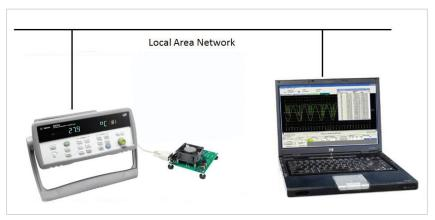
Figure 1. The Agilent 34972A data acquisition instrument takes measurements remotely over LAN
