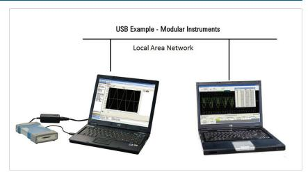
Figure 6. The Agilent U2700A USB-Enabled modular instrument accessed via remote pc-to-pc connection
