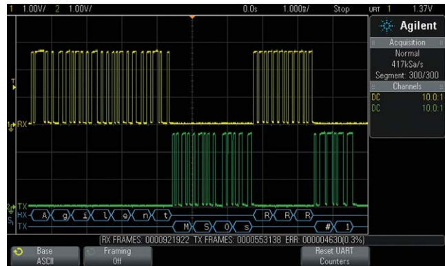
Figure 13. RS-232 protocol analysis on a 3000 X-Series oscilloscope
