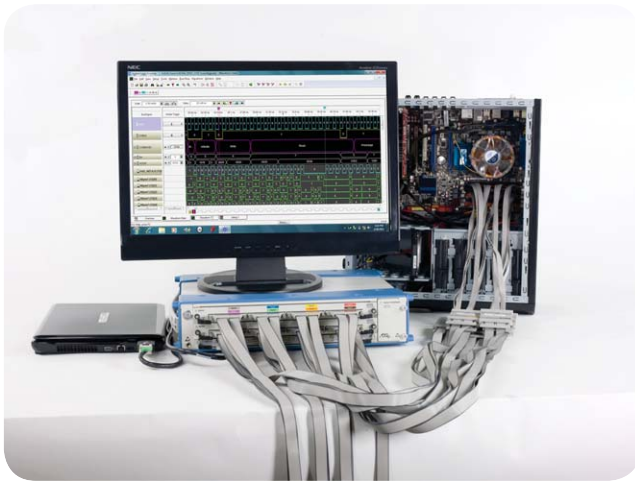
Figure 6. U4154A-4 Gb/s DDR3 logic analyzer solution
