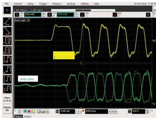
Figure 4. Using InfiniiScan software's zone qualify trigger enables you to trigger on read or write bursts to separate read and write data for eye diagram testing. Read data is edge aligned with the strobe while the write data is center aligned with the strobe.
