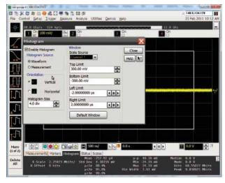
Figure 3. Histogram measurement window for an Agilent oscilloscope
