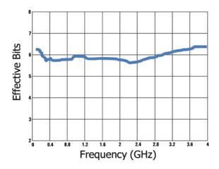
Figure 5. Shown here is sample ENOB plot for Agilent's Infiniium 9000 Series oscilloscope. The plot represents ENOB for the entire scope system and not just its 8-bit ADC.
