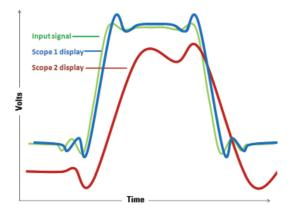
Figure 8. Scope 1 and 2 have the same ENOB, but scope 2 has offset and phase distortion errors that limit its ability to correctly display the input signal.
