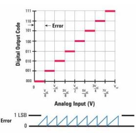
Figure 6. The magnitude of the error ranges from zero to 1 LSB
