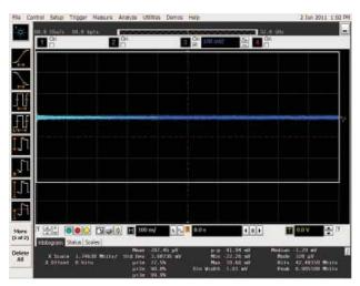
Figure 4. The offset can be changed by adjusting the signal up one division
