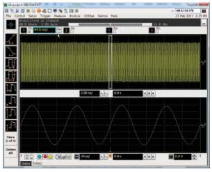
Figure 7. Applying the sine wave to a channel and frquency produces this waveform
