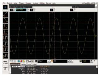
Figure 1. Noise influences oscilloscope jitter, as seen by looking at the time-interval error for various sine-wave frequencies.
