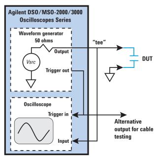
Figure 1. Test configuration
