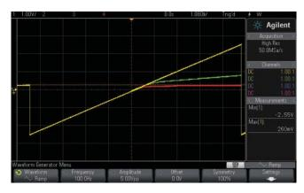
Figure 4. Diode and transistor measurement: without a DUT connected (yellow trace); with a small signal silicon diode as the DUT (green trace); with a power Schottky diode as the DUT (red trace).
