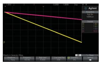
Figure 5. Output resistance measurement: without a DUT connected (yellow trace); with a 74ACT08 DUT attached (red trace).
