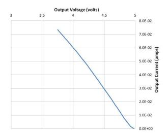
Figure 6. Measured load line for a 74ACT08 logic gat output.
