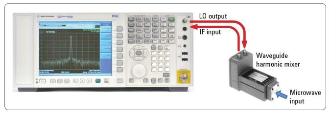
Figure 1. External mixing, shown here with the Agilent PXA signal analyzer, moves the first mixing (downconversion) stage outside of the analyzer by sending an external mixer a tuned LO signal and bringing an IF signal back in. Further signal processing is similar to internally-mixed measurements.
