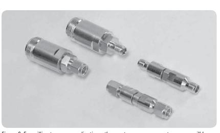
Figure 6. For millimeter-wave applications, the most common connector savers will have female connectors on both ends. Shown here are adapters to connect an analyzer with 2.4 mm front panel connectors to type-N and 2.4 mm accessories.
