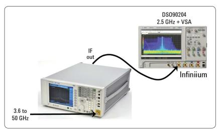
Figure 3. Agilent PXA signal analyzer is used as a wideband downconverter. IF bandwidths as wide as approximately 900 MHz are available for digitizing with external solutions such as oscilloscopes. Signal processing for spectrum, vector, and demodulation measurements is performed by Agilent 89600 VSA software in the oscilloscope or a host PC.
