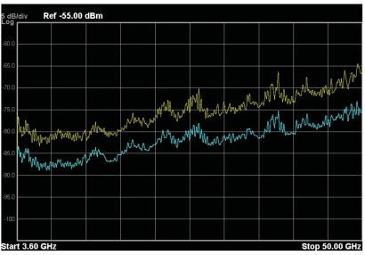
Figure 8. This measurement covering 3.6 to 50 GHz at 5 dB/div illustrates the noise floor improvement when the PXA low noise path is selected.
