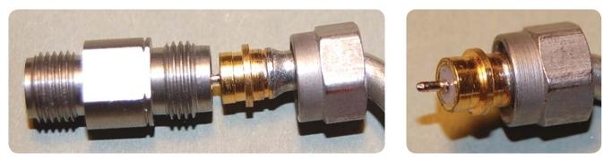
Figure 7. Figure 7a shows a 2.4 mm-to-3.5 mm adapter with the 2.4 mm end of the adapter on the right. The male connector at right is an SMA. The SMA male connector in Figure 7b has a non-captive nut and a male conductor which is displaced axially (too long) and is slightly bent, perhaps from the bending of the semi-rigid cable adjacent to the connector.
