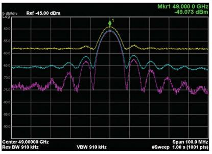
Figure 9. Measurements of this low level signal at 49 GHz are improved significantly through the use of the low noise path and noise floor extension features of the Agilent PXA. The top trace is a normal measurement, the middle trace is made with the low noise path selected, and the bottom trace shows the benefit of adding the noise floor extension feature.
