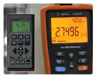
Figure 4. Inaccurate VFD output frequency measurement without low pass filter
