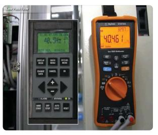
Figure 5. Accurate VFD output frequency measurement with low pass filter
