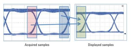
Figure 10. More effectively using the acquired samples to quickly create and display the eye diagram.
