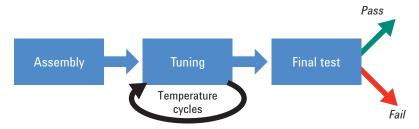
Figure 2. Typical manufacturing flow for more complex devices.
