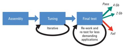
Figure 1. Typical manufacturing flow for simpler and less expensive devices.
