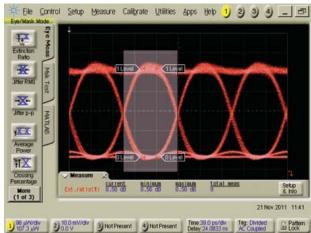
Figure 8a and b. Eye diagrams showing the typical region of samples used to calculate measurement results without Rapid Eye.
