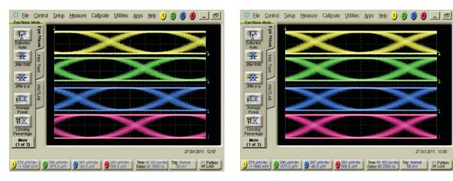
Figure 4a and b. Typical eye diagrams where eyes are not aligned and are aligned.
