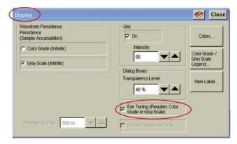
Figure 6. Display dialogue box to enable Eye Tuning mode.
