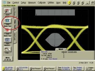
Figure 15. Acquire all samples, then apply the mask test.
