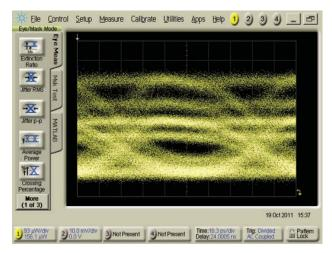
Figure 5. Typical eye display when tuning a laser.
