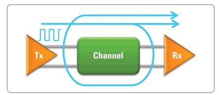
Figure 1. Multiple reflection between transmitter and receiver
