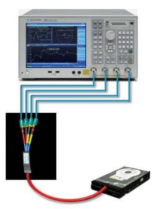
Figure 9. Hot TDR measurement example for SATA HDD
