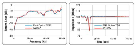
Figure 6. Correlation between 86100D TDR oscilloscope and ENA Option TDR for return loss (left) and impedance (right) measurements
