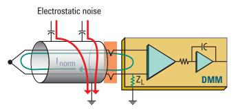
Figure 3: Stray capacitance can couple electrostatic noise through a thermocouple.
