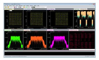
Figure 2. 3-channel 802.11ac analysis using Agilent's 89600 VSA software.
