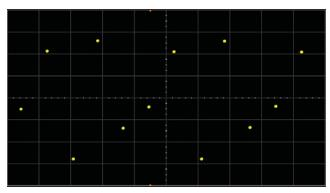
Figure 1: Single-shot capture of a 1-GHz sine wave sampled at 2.5 GSa/s, but without digital waveform reconstruction filtering.
