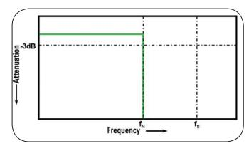
Figure 7: Theoretical brick-wall frequency response.
