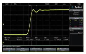
Figure 4: Capturing a fast rising edge at 2.5 GSa/s with automatic sin(x)/x waveform reconstruction.
