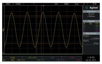
Figure 2: Single-shot capture of a 1-GHz sine wave at 2.5 GSa/s with sin(x)/x reconstructed samples.
