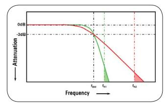
Figure 8: Typical oscilloscope frequency responses.
