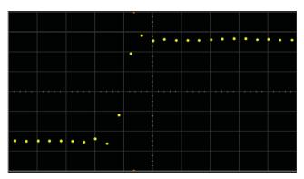
Figure 3: Single-shot capture of a fast rising edge sampled at 2.5 GSa/s, but without digital waveform reconstruction filtering.
