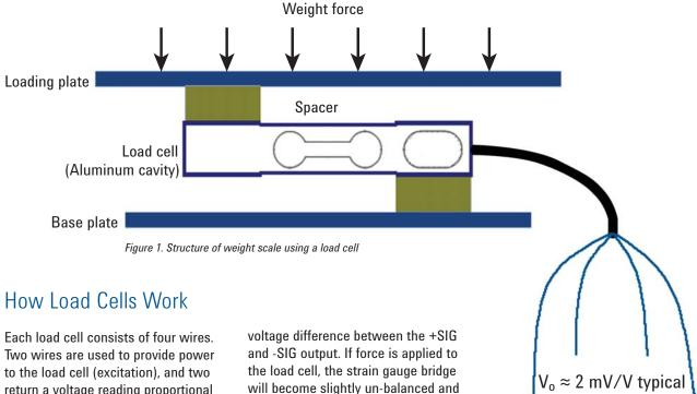
Each load cell consists of four wires. Two wires are used to provide power to the load cell (excitation), and two return a voltage reading proportional to the weight on the cells (signal). There are many varieties of load cells on the market, strain gauge-based load cells are the most commonly used. A strain gauge is a thin strip of metal designed to measure mechanical load by changing resistance when stretched or compressed within its elastic limits.
