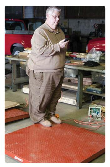
Figure 3. Identify a bad load cell with corner testing
