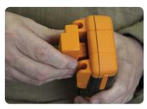
Figure 4: Attaching Agilent U1177A IR-to-Bluetooth adapter to the Handheld Multimter
