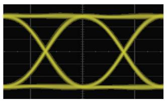
Figure 1: Capturing DDR2-667 data signals using an Agilent 500-MHz bandwidth scope.
