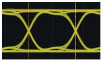
Figure 2: Capturing DDR2-667 data signals using an Agilent 1-GHz bandwidth scope.
