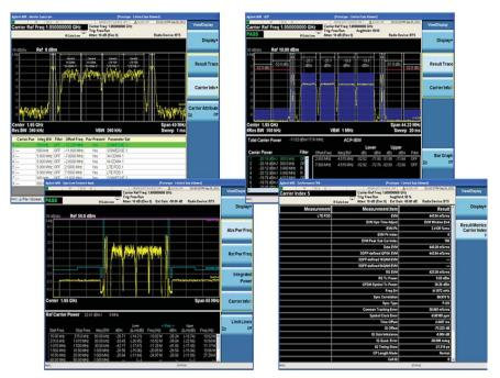
FIGURE 2. As a 3GPP-dedicated MSR signal analysis application, the N9083A MSR measurement application enables fast one-button measurements per 3GPP TS37.
