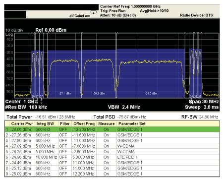
FIGURE 3. Shown here is a swept-spectrum view of a carrier-channel power measurement for one of the MSR conformance testing defined in 3GPP TS37.141.
