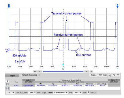
Figure1: GPRS smart phone active mode current drain waveform details.
