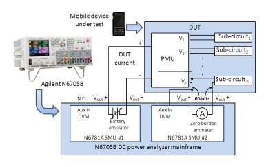
Figure 2. Battery input and subcircuit power test setup using Agilent N6781A source/measure units
