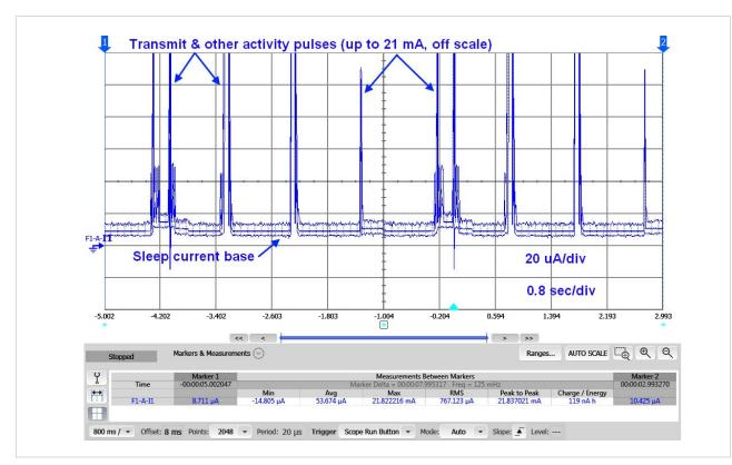
Figure 2: Wireless temperature transmitter current drain, seamless ranging measurement
