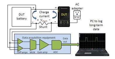
Figure 1. Traditional battery charge profile measurement test setup
