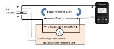
Figure 2. Battery run-down test setup using the Agilent N6781A source/measure unit
