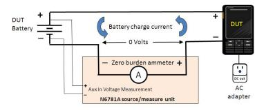
Figure 2. Battery charge profile test setup using the N6781A source/measure unit.
