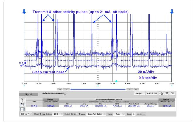
Figure1: Wireless temperature transmitter current drain, fixed ranging measurement
