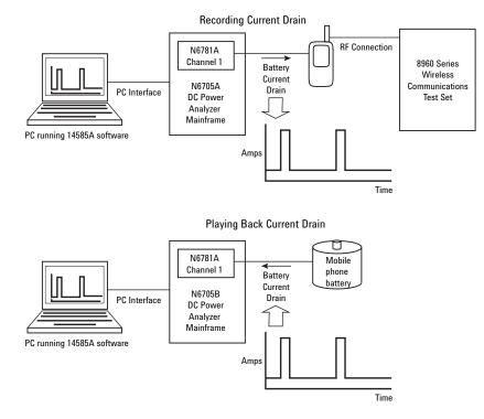
Figure1. Recording and playing back a device's current drain to discharge a battery.
