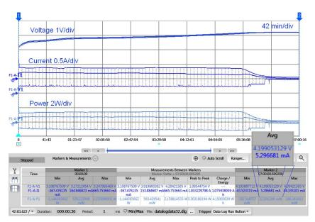
Figure 3. Battery charge profile measurement test results.
