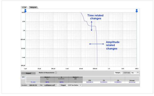
Figure1: CCDF profile of a mobile phone's standby current drain
