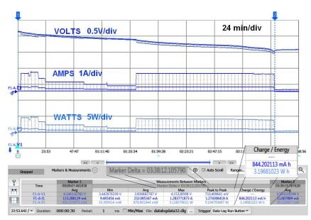
Figure 3. Battery run-down test results
