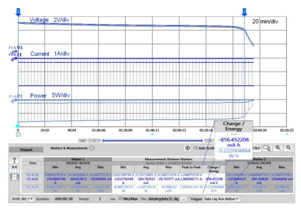
Figure2. Measuring battery capacity under end-use pulsed loading condition.
