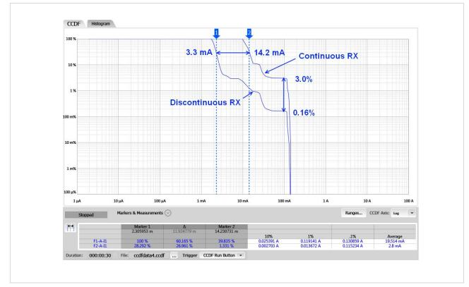
*Figure 2: Analyzing a mobile phone's standby power savings details using CCDF profiles* 10
