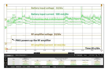
Figure 3. Battery input and subcircuit power test results on a GPS device
