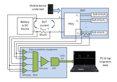
Figure 1. Conventional battery input and subcircuit power test setup
