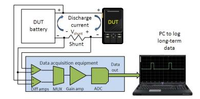
Figure 1. Conventional battery run-down test setup
