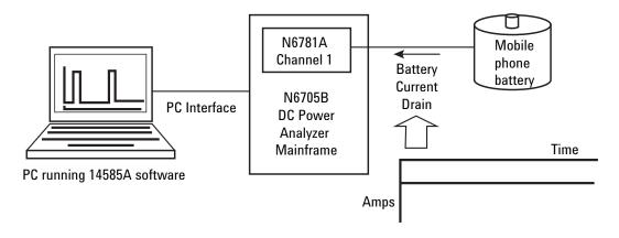
Figure1: Using a constant current load to discharge a battery at a fixed C rate.
