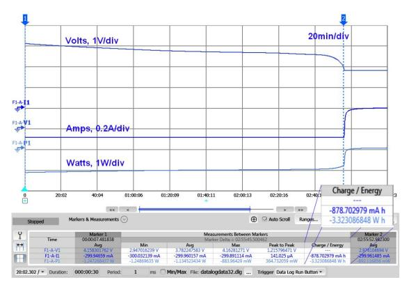
Figure2: Measuring a battery's capacity and energy using the 14585A software.
