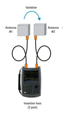
Figure 6b. Configuration for measuring antennato-antenna isolation
