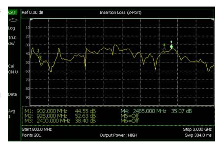
Figure 7. Measured antenna-to-antenna isolation between a 900-MHz panel antenna to a 2.4-GHz panel antenna mounted on the same structure
