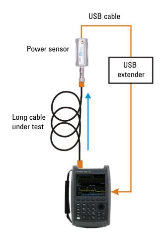
Figure 4. Configuration for measuring cable loss using FieldFox and a USB power sensor
