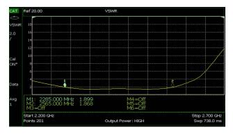
Figure 5a and 5b. Frequency response measurement of a panel antenna showing (a) return loss (dB) and (b) VSWR
