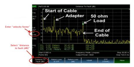
Figure 9. Measurement of the distance-to-fault (dB) for the configuration shown in figure 8
