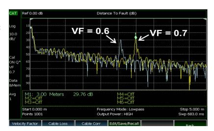
Figure 13. Measurement of a Category-6 patch cable with adjustment to FieldFox's velocity factor correction in order to match the measured distance to the known physical distance
