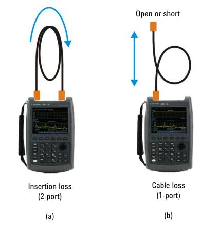
Figure 2. Configurations for measuring the insertion loss of a cable using FieldFox with CAT mode
