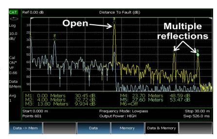
Figure 10. DTF measurement comparison between cable terminated in open circuit (yellow) and 50-ohm load (blue)
