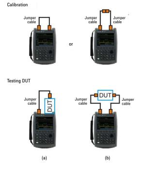
Figure 15. Configuration for the Normalization Cal Type using a jumper cable(s) required for 2-port insertion loss testing of a DUT
