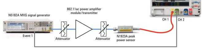
Figure 2. 802.11ac transmitter power measurement setup diagram
