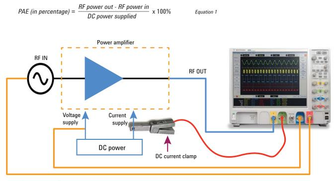
Figure 6. Power added efficiency test setup
