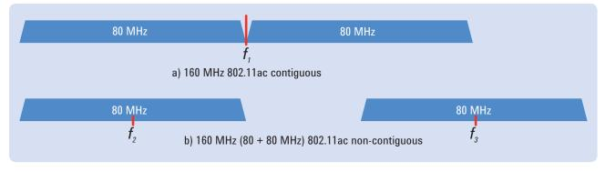
Figure 1. 802.11ac 160 MHz bandwidth channelization
