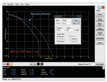
Figure 5. 802.11ac CCDF plot obtained using an 8990B PPA
