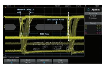
Figure 4: CAN eye-diagram mask test on a 500 kbps differential bus viewed in a dominant-bit-low format.
