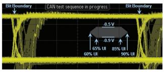
Figure 9: Pass/Fail mask for an 80 meter network operating at 500 kbps.
