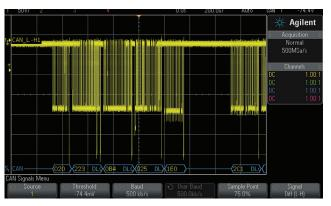
Figure 3: Probing the differential CAN bus to show dominant-bit-low.
