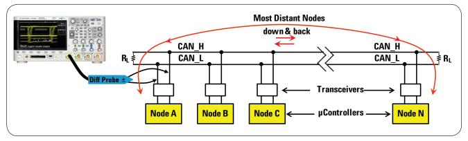
Figure 6: Typical multi-node CAN network.
