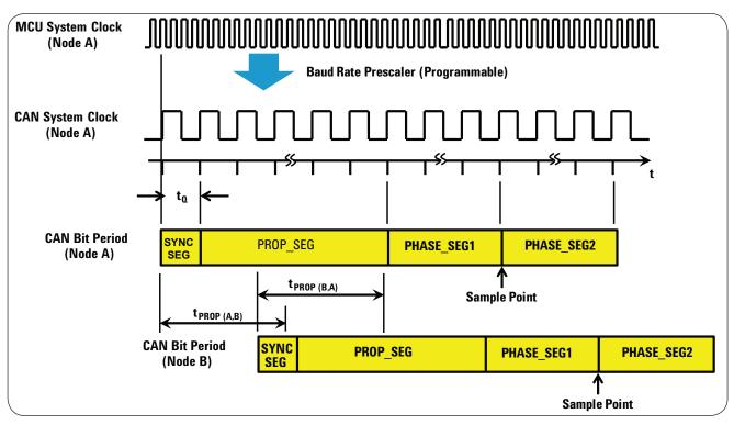
Figure 5: CAN bit-timing diagram for two widely-spaced nodes.
