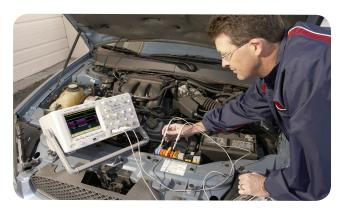
Figure 9: The Agilent 6000 Series oscilloscope with battery and automotive bus options.
