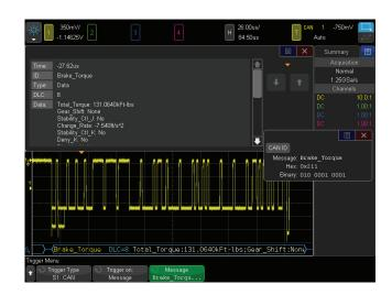
Figure 3: CAN-dbc symbolic decode and trigger.
