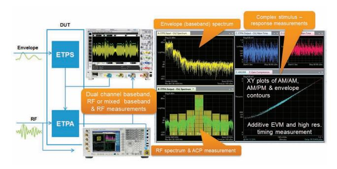
Analyze both RF and envelope signals using the 89600 VSA software
