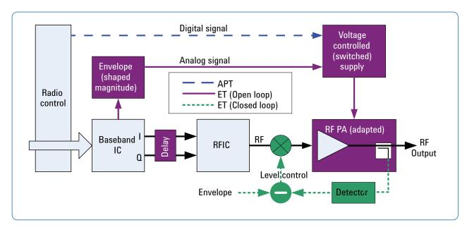
In a practical system, the envelope signal may be generated in the RFIC.
