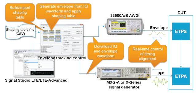
Synchronous envelope and RF signal generation
