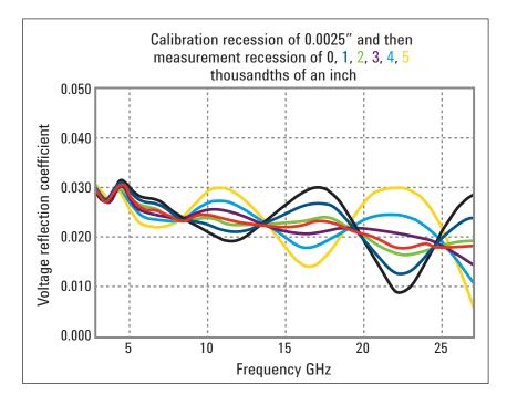
In *Figure 6*, recession during calibration was set midway between the extremes of recession for measurement. This produced a plot that resembles an amplitude-modulated signal and clearly shows the combination of the plots from *Figures 4/5*.
