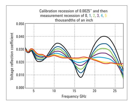
*Figure 5* is similar to *Figure 4* but with the errors "reversed". With 0.005" recession during calibration then zero recession during measurement, the effect is similar to that for a connector with protrusion (providing the test port has sufficient recession to avoid damage). However, the peaks occur where the troughs were positioned in the previous chart.
