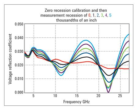
*Figure 4* shows an ideal calibration performed with no recession and the measured load adjusted in 0.001" increments from zero to 0.005". At approximately 22 GHz it is apparent that the predictability of the results changes. As the recession continues to increase, the VRC reaches a minimum and starts to return towards its original value.
