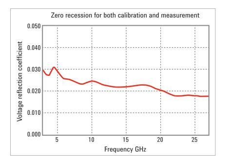
*Figure 2* forms the reference for the following measurements and is shown on all plots as the red line. It was performed with both the calibrating and measured sliding load set to zero recession. This is considered to be the correct representation of the voltage reflection coefficient (VRC) of the tested sliding load.
