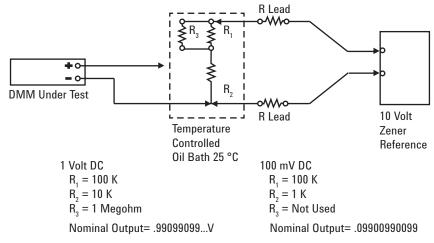
Figure 1. (Loading Corrections Must Be Made When Using Dividers)
