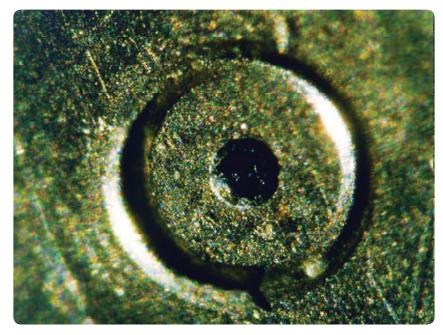
Extreme fiber damage on connector.
