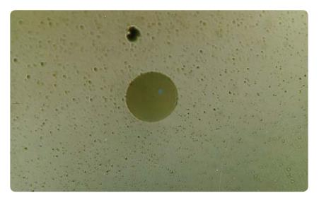
Again cleaned with isopropyl alcohol in some way but compressed air blown over ferrule end.
