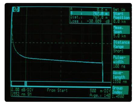
Typical result of damaged front panel connector
