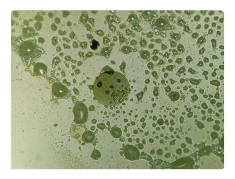
Isopropyl alcohol (IPA) applied with cotton bud and cleaned, waved in air to evaporate IPA.
