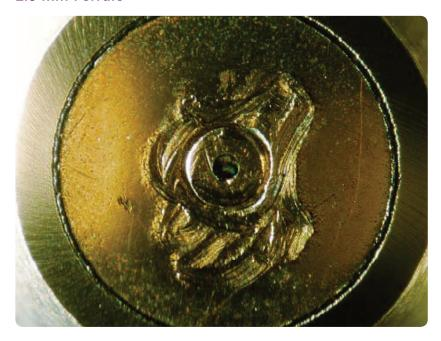
Assume that ferrule end was 'cleaned' by probing with pin.
