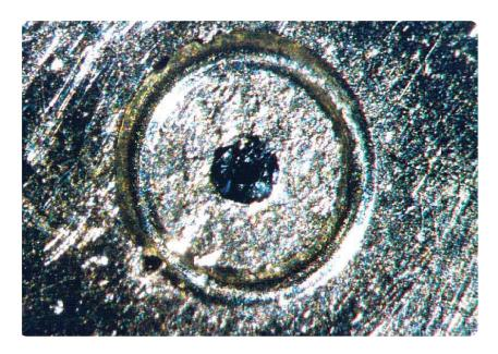
Multimode fiber with 62.5  $\mu m$  core and 125  $\mu m$  cladding diameter (black and dark blue, respectively).
