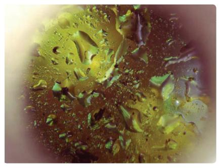
Picture through front panel connector of collimating lens. User has attempted to remove RI liquid with solvent.
