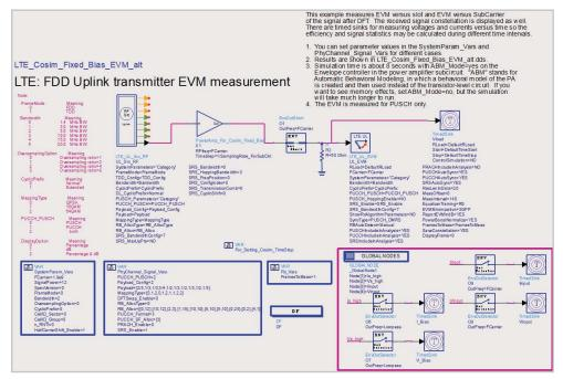
Figure 25. LTE Cosim Fixed Bias EVM alt co-simulation schematic.
