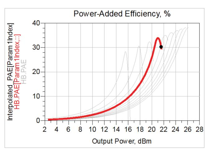
Figure 7. Plot of PAE versus output power, showing increasing drain bias from left to right.
