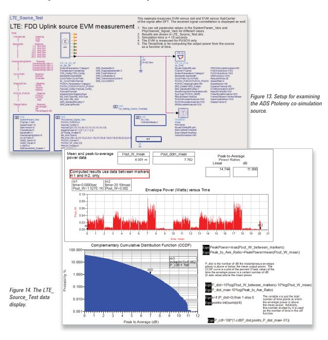
The test signal has bursts of different power levels, leading to a high PAPR. Moving the markers on the display shows power data within a particular burst. Alternatively,
