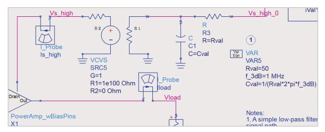
Figure 40. Schematic for simulating finite bandwidth in the bias modulation signal path.
