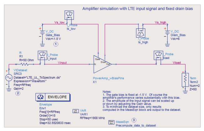
Figure 16. Simulating the power amplifier with a fixed drain bias.
