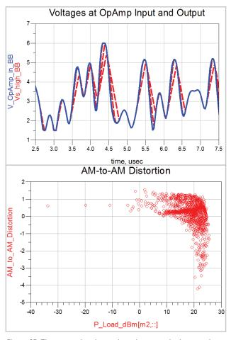
Figure 35. The upper plot shows the voltages at the input and output of the OpAmp, while the lower image shows a large AM-to-AM distortion.
