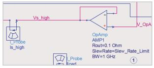
Figure 33. Schematic for modeling effects of a finite slew rate in the bias modulator.
