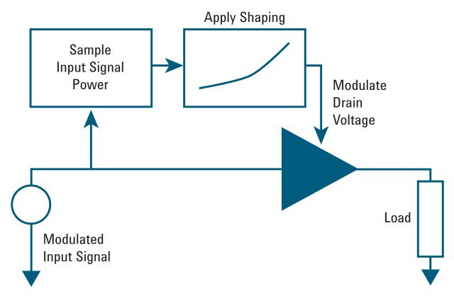
Figure 3. A block diagram for simulating Envelope Tracking.
