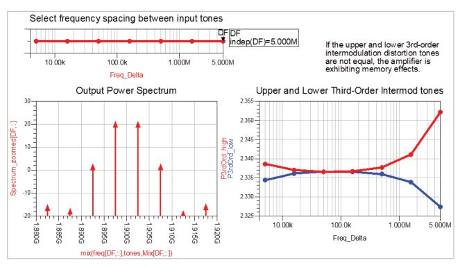
Figure 5. Simulation results for the example of a PA designed for wideband modulation.
