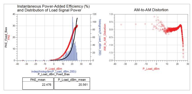
Figure 22. ET simulation using a shaping table to maintain 11 dB constant gain.
