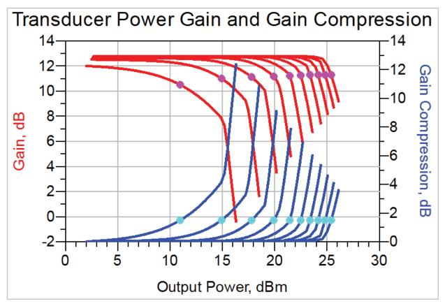
Figure 11: Interpolated values at 1.5 dB of gain compression.
