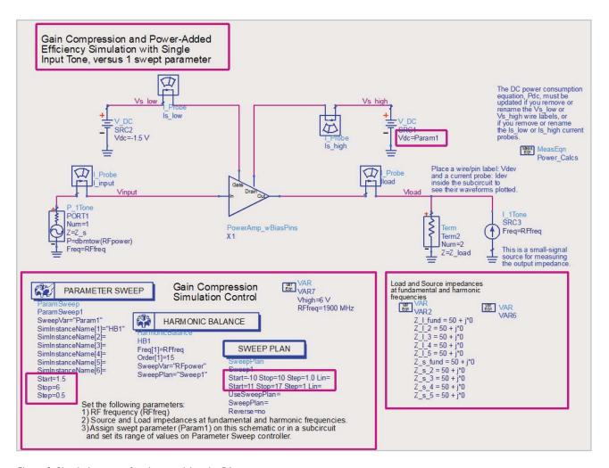
Figure 6. Simulation setup for characterizing the PA.
