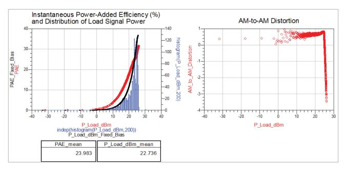
Figure 21. ET simulation with Gain=2.5 on the LTE source.
