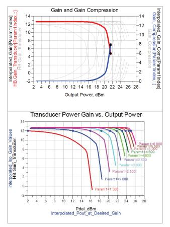
Figure 8. Plot of gain and gain compression.
