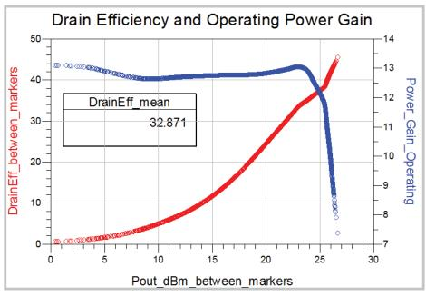
Figure 30. Drain efficiency and operating power gain during the 7 to 8 msec. burst, with ET on.
