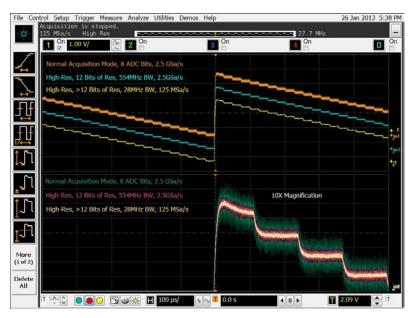
Figure 3. High-resolution signal trace examples
