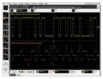
Figure 6. High resolution works great for capturing a low-noise PRBS signal, while averaging does not
