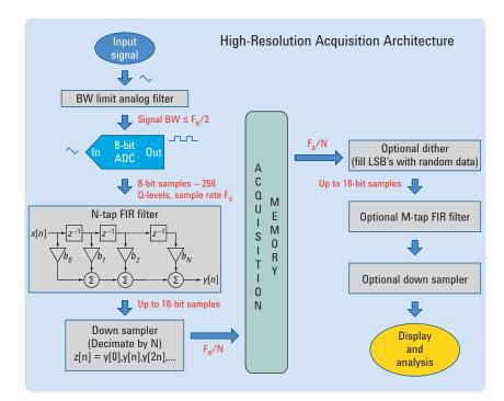
Figure 4. High-resolution acquisition architecture
