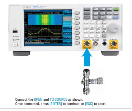
Figure 3. Performing OSL calibration on the N9322C BSA
