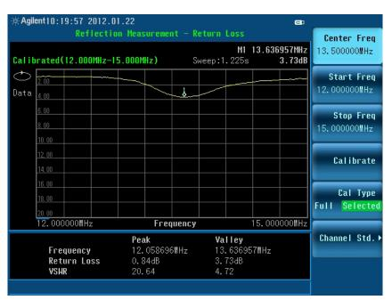
Figure 5. Return loss result measured with the N9322C BSA
