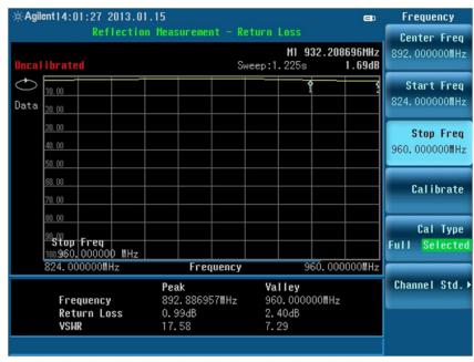
Figure 5. Reflection measurement mode waiting for OSL calibration
