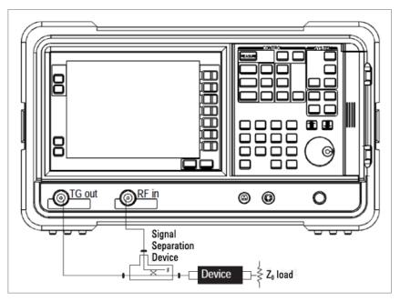
Figure 2. Conventional test setup requires an external bridge
