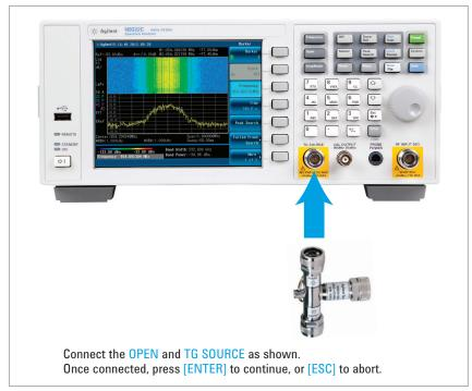
Figure 6. Performing open-short-load calibration on the N9322C BSA
