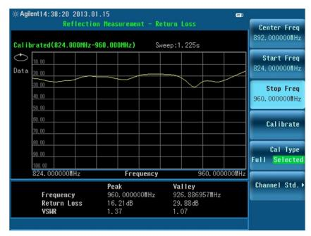
Figure 8. A calibrated return loss measurement across the selected frequency range
