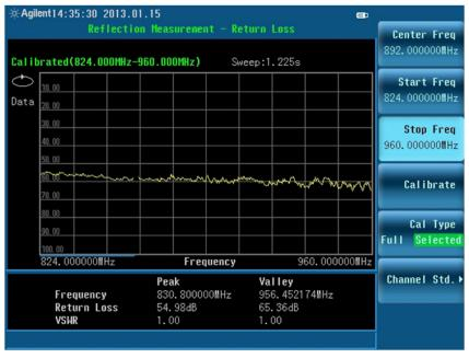
Figure 7. The calibrated N9322C BSA ready for measuring return loss/VSWR
