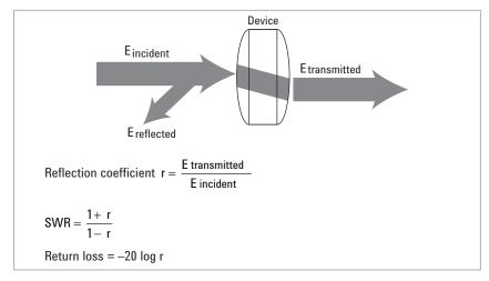
Figure 1. Reflection measurements
