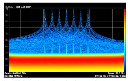
Figure 3. The density or histogram display collects a large amount of real time spectrum data into a single display that shows both rare and frequent events, with an indication of relative frequency of occurrence.
