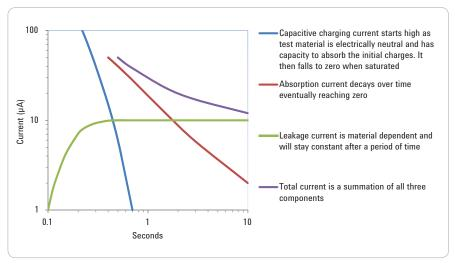
Figure 1. Components of test current
