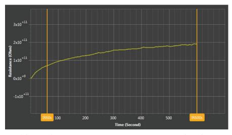
Figure 2. Curve plot of a time-resistance test made on a motor winding, using test software. Good insulation shows a continual increase in resistance, in inverse exponential trend
