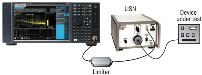
Figure 4. Conducted measurements interconnection
