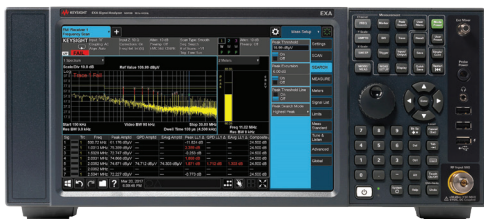
X-Series analyzer with N6141C EMC measurement application
