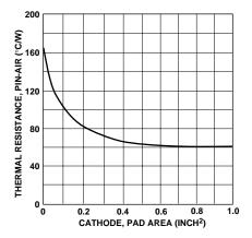
Figure 1. Printed Circuit Thermal Resistance  $(\theta_{P-A})$
