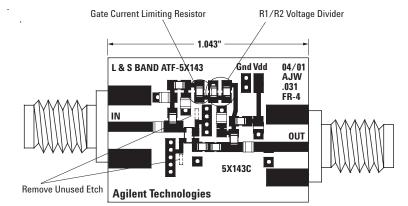
Figure 2. 5X143C Demo Board with Components Installed. Note location of PHEMT bias resistors R1 and R2.
