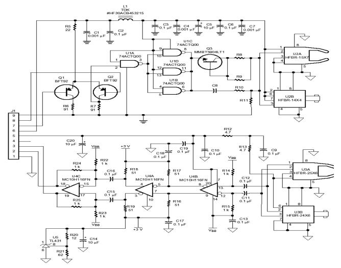
Figure 2. Cost-Effective 160 MBd Fiber Optic Transceiver.
