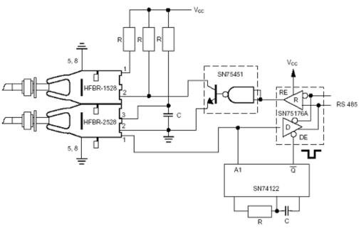
Figure 1. Basic RS-485 Fiber Optic Interface Adapter to Data Terminal.
