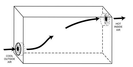
Figure 1. Use of Fans to Augment Convection Cooling.
