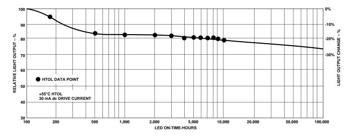
Figure 1. Projection of Statistical Average Light Output Degradation Performance for AS AlInGaP LED Technology to 100,000 Hours, extrapolated from 10,000 hour HTOL data.
