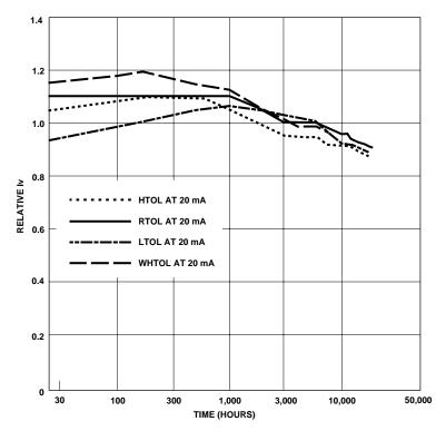
Figure 1. AlInGaP Light Output Degradation Data at 16,000 hours for Various Environmental Conditions. Lamps Under Test are stressed and tested at 20 mA dc. Light Output Data is measured at 25°C, referenced to Time Point Zero.
