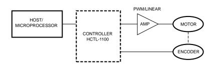
Figure 1. Closed Loop Position and Velocity Control of DC Brush Motor
