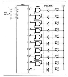
Figure 8. BCD to 10 Element Bar Graph Array
