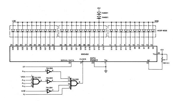
Figure 9. Serial Data Interface Between 6800 and 30 Element Bar Graph Array
