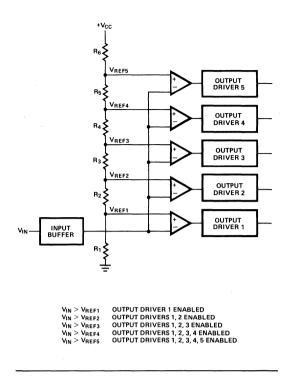
Figure 3. Typical Analog Input Bar Graph Decoder
