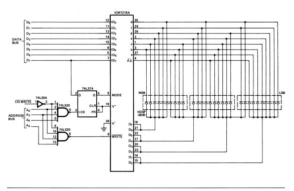
Figure 11. Parallel Data Interface Between 8080A and 30 Element Bar Graph Array
