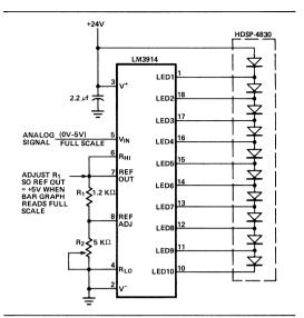
Figure 6. Low Power 0V-5V Bar Graph Meter
