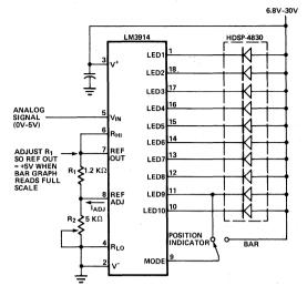
Figure 5. 0V-5V Bar Graph/Position Indicator Meter
