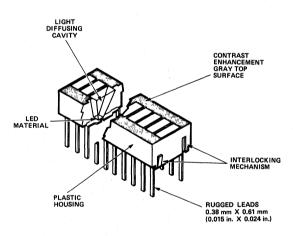
Figure 1. 10 Element Bar Graph (Cutaway)
