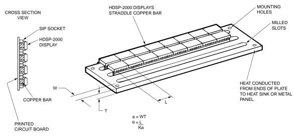
Figure 28. Multiline HDSP-2000 Heat Sink
