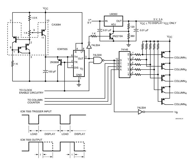
Figure 31. Wide Range Intensity Modulation Control and Power Switching of Display I<sub>CC</sub> to Conserve Power
