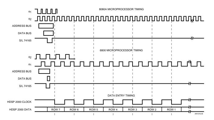
Figure 5. REFRESH CONTROLLER Timing
