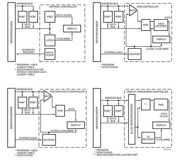
Figure 3. Four Different Techniques to Interface the HDSP-2000 Alphanumeric Display to a Microprocessor System
