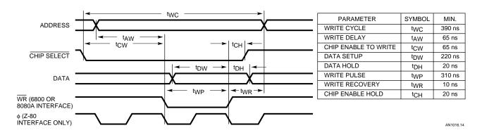
Figure 14. Memory Write Timing for the 32 Character HDSP-2000 CODED DATA CONTROLLER
