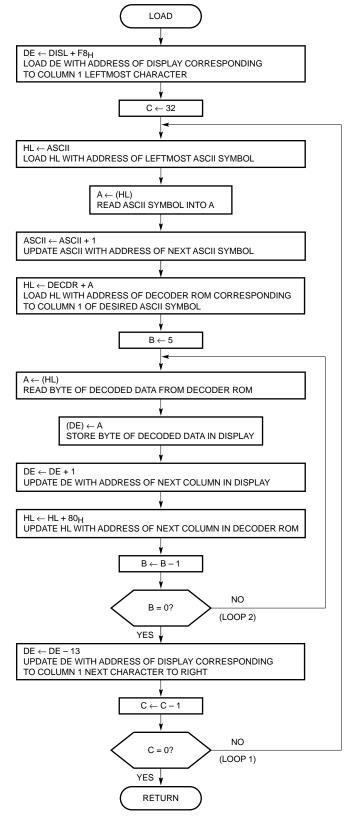
Figure 12. 8080A Microprocessor Program that Decodes a 32 Character ASCII String Prior to Loading into the DECODED DATA CONTROLLER
