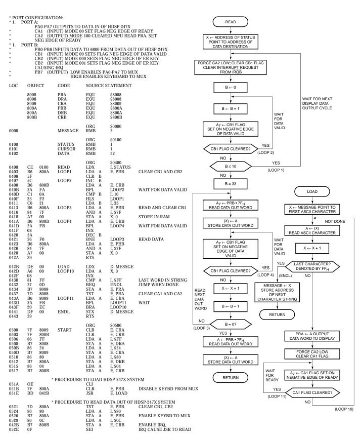
Figure 21. 6800 Microprocessor Program that Interfaces to the Circuit shown in Figure 14.
