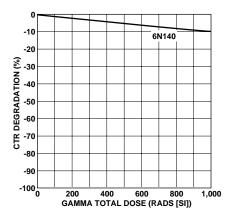
Figure 3. Agilent Optocoupler Gamma Radiation Response
