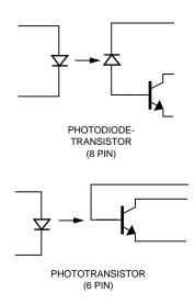
Figure 2. Photodiode and Phototransistor Optocoupler Schematics
