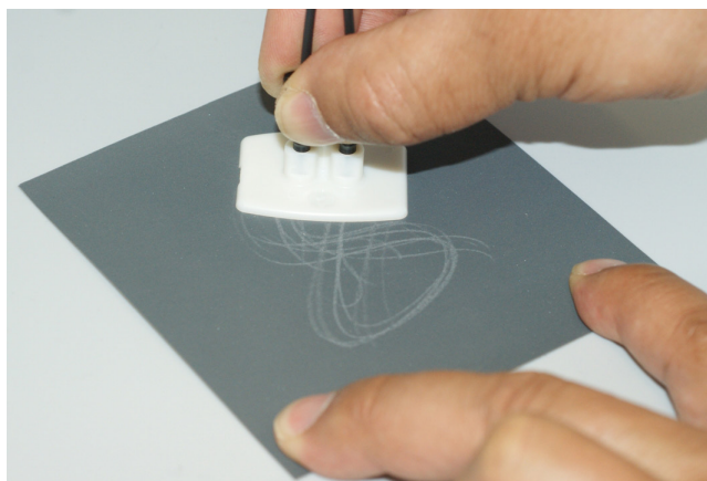
Figure 27. Polishing by drawing pattern 8 on abrasive paper
