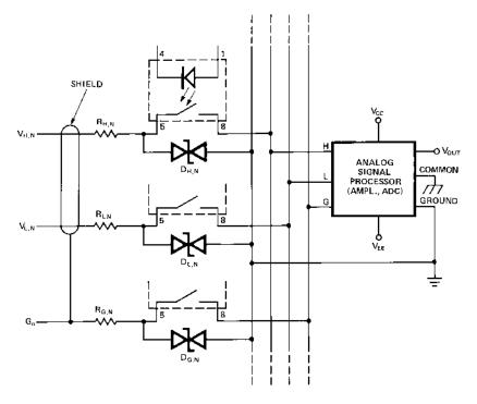
device can be used up to the FULL withstand voltage of the open contacts.
