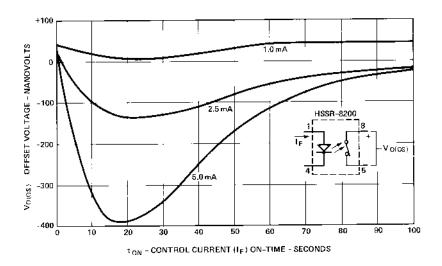
Figure 13. Typical Contact Offset Voltage.
