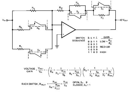
Figure 5a. Inverting Amplifier Gain Switching.
