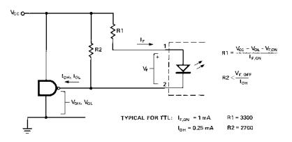
Figure 7. Logic-Driven Control Circuit.
