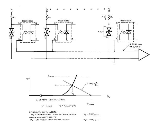
Figure 14. Over-Voltage Protection in Multiplexer Application.
