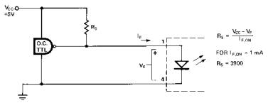
Figure 8. Shunt-Driven Control.
