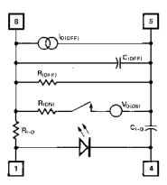
Figure 3. Approximate Equivalent Circuit of HSSR-8200.
