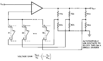
Figure 5b. Non-Inverting Amplifier Gain Switching.
