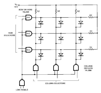
Figure 10. Matrix-Driven Control Circuit.
