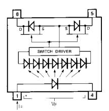
Figure 2. Circuit Diagram of HSSR-8200.
