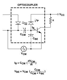
Figure 8. Common-Mode Interference Model.
