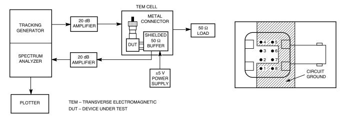
Figure 3. Block Diagram of Test Setup for Electromagnetic Susceptibility
