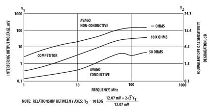
Figure 2. Typical Output Signal Due to 10 V/m Field with Metal Ferrule
