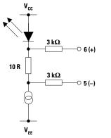
Figure 4. Bias Monitor External Connections for HFCT-5201 listed in Table 1
