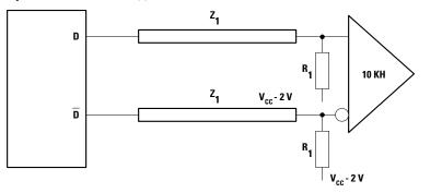
Z<sub>1</sub> = 50 ohms Interconnect R<sub>1</sub> = 50 ohms
