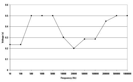
Figure 8. HFCT-5205/HFCT-5103/HFCT-5201/HFCT-5215 Tolerable Receiver Injected Power Supply Noise Amplitude versus Frequency without Power Supply Filtering
