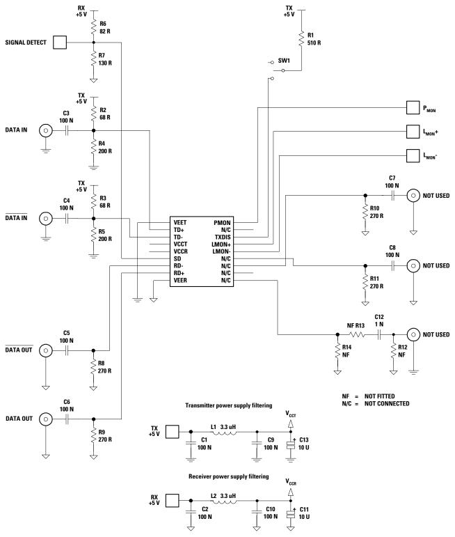
Figure 11. HFCT-5000 Evaluation Board Schematic
