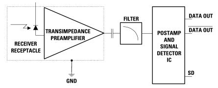
Figure 6. Simplified Receiver Schematic
