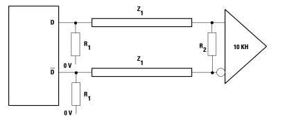
$\begin{array}{l} Z_1 = 50 \text{ ohms Interconnect} \\ R_1 = 270 \text{ ohms} \\ R_2 = 100 \ \Omega \end{array}$
