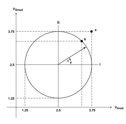
Figure 1. I and Q coordinate axes. "a" is the point where peak output power is measured. "b" is the point where the SSB output power is measured.
