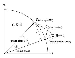
Figure 2. Illustration of error vector magnitude for calculating percent modulation error.
